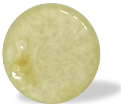
Figure 2. PIM membrane with Poly-BADGE 2:1 carrier.
